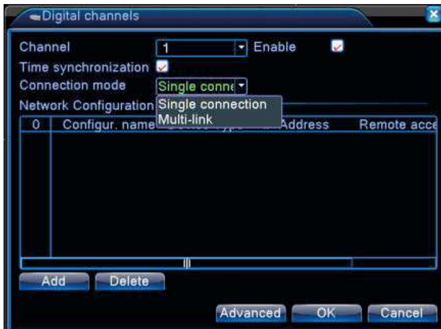
Pic 2.3.3 single link page and multi-link page of digital channel
