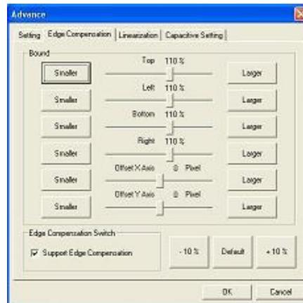
In some case, if it is difficult to touch items at the edges of the touch panel, users can set adjustment to reach the edges of the screen image.
