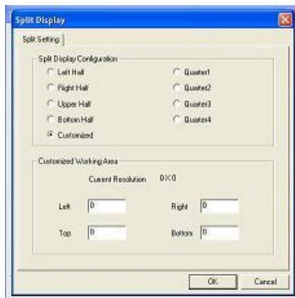
It shows the current resolution of display and users can set up the activate area by inputting the value by yourself or use the default button.
