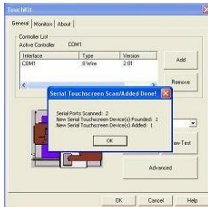
The controller is displayed on the Panel List box. Users can get the information of interface, type, firmware version and baud rate for each controller.
